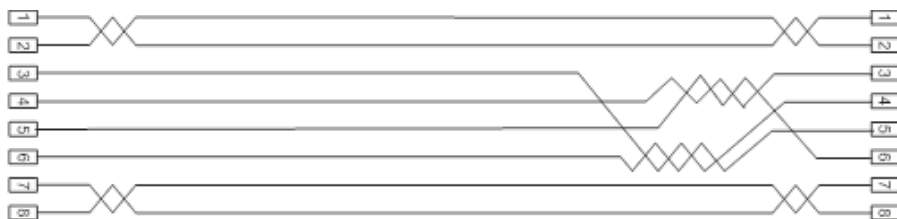
BRI ISDN Cable cross TE configuration
