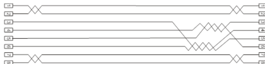
BRI ISDN Cable cross TE configuration
