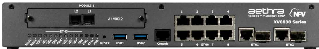
Fig. 5: XV8800VE2WAC / XV8800VE2LWAC uCPE with VDSL2 35b bonding.
